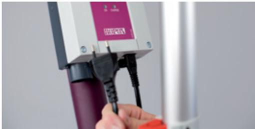
Recharging is simply done by plugging the power cord into the wall socket.
